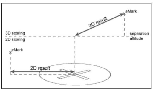
When goals/targets above the ground are used, result based on track points will be the 3D distance.
